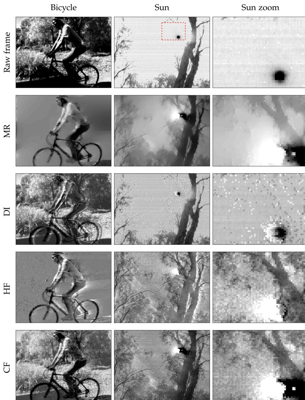
Figure 3.6: **Sun**: Raw frame is overexposed when pointing directly at the sun (black dot is a camera artifact caused by the sun). In MR, some features are smoothed out (see zoom). DI is washed out due to the latest frame reset. CF captures detailed leaves and twigs. **Bicycle**: Static background cannot be recovered from events alone in MR and HF. CF recovers both background and foreground.
